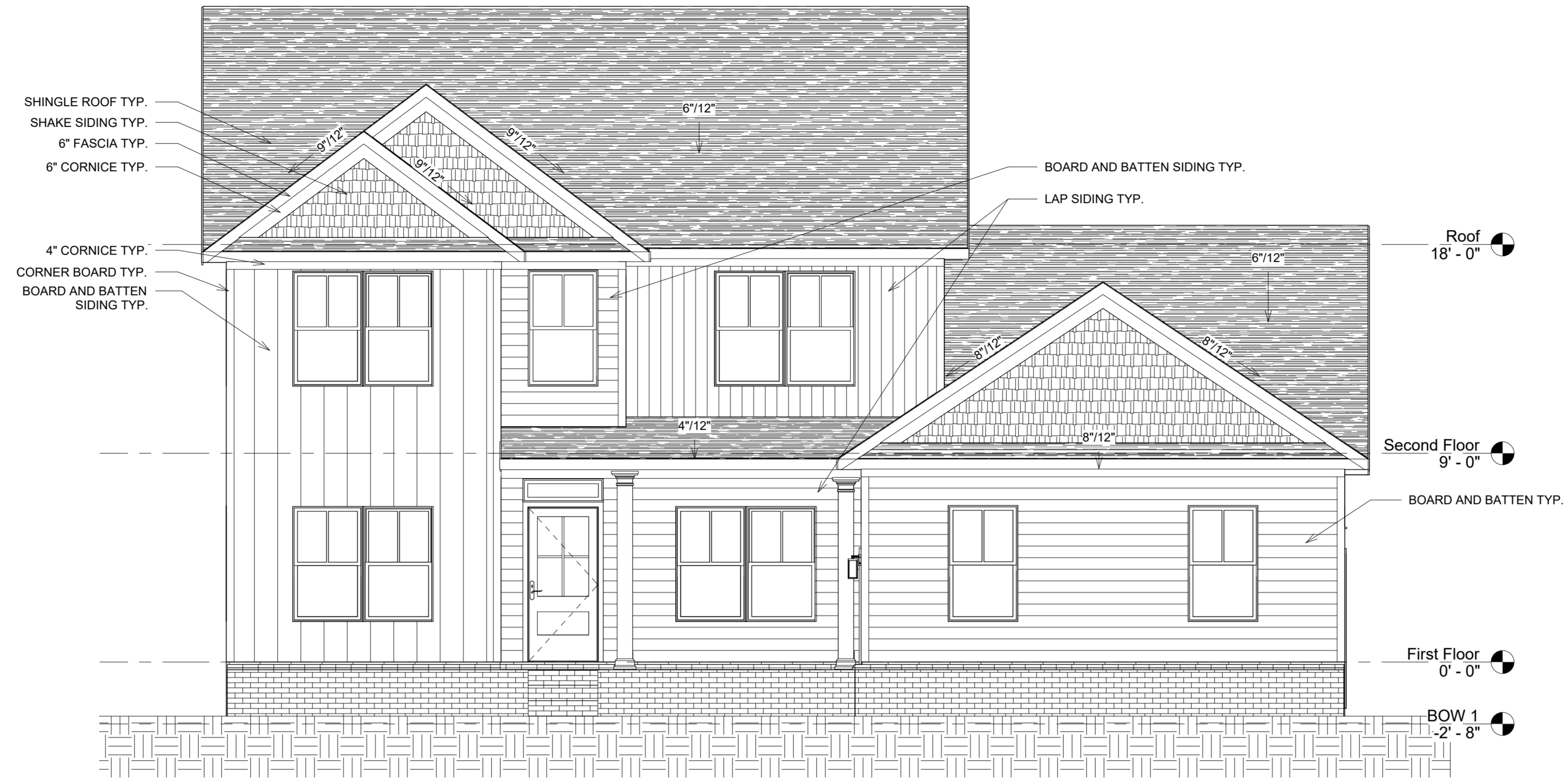
① South Elevated Slab Opt. Back Porch 1/4" = 1'-0"
