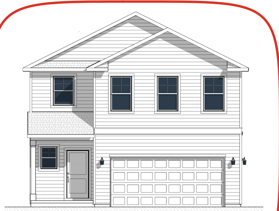
1 FRONT ELEVATION - A CS CS-1 1/8" = 1'-0" WHEN PRINTED ON 11"x17" / ANSI B PAPER SIZE 1/4" = 1'-0" WHEN PRINTED ON 22"x34" / ANSI D PAPER SIZE
