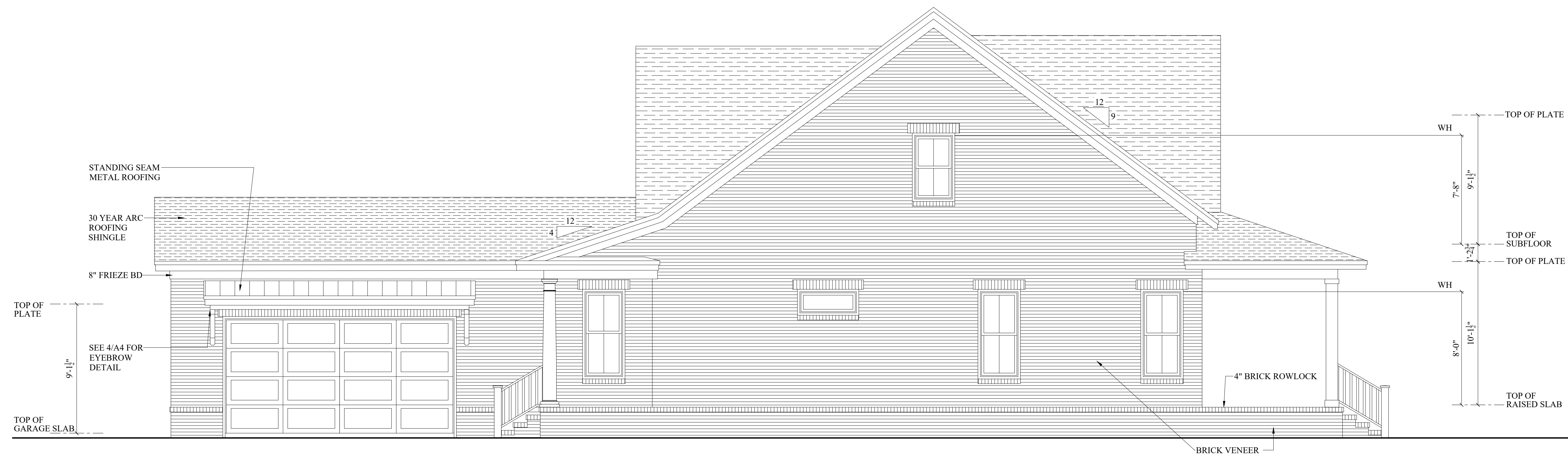
2 RIGHT SIDE ELEVATION 1/4"=1'-0"
